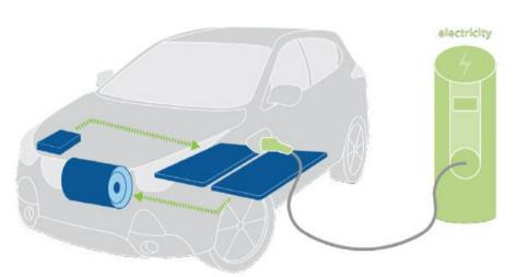
that powers one or more electric motors. Battery electric vehicles run entirely on the energy stored on an onboard battery. The vehicle is charged by electricity from the grid. On average, the vehicle's range is upwards of 80 miles on a single charge. BEVs can be plugged in at home, work or public charging stations. In addition, there is limited maintenance: the vehicle will never require an oil change.
